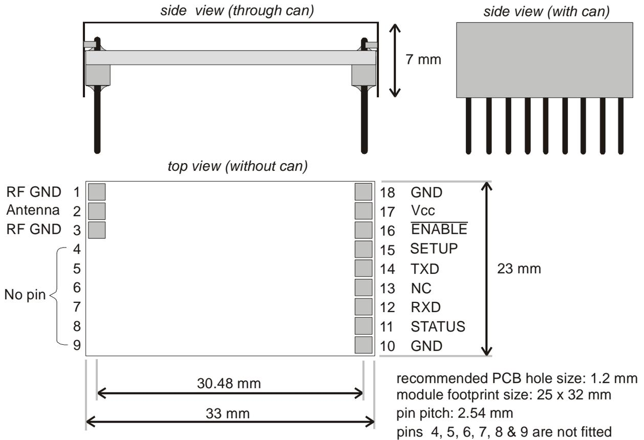
**Figure 3: TDL2A footprint (top view)**
