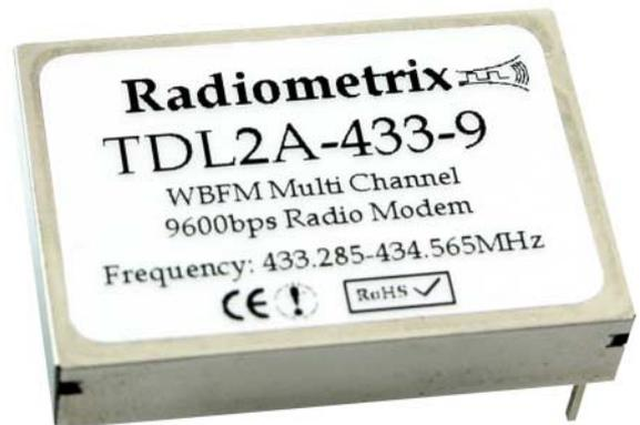
Figure 1: TDL2A-433-9 radio modem
