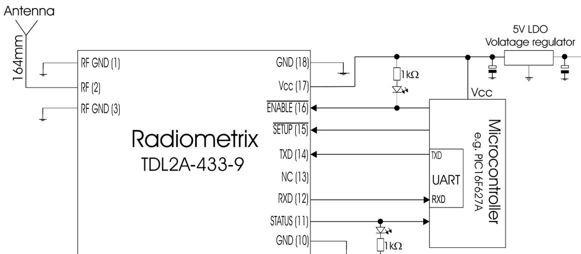
**Figure 6: TDL2A interfaced directly to a microcontroller**
