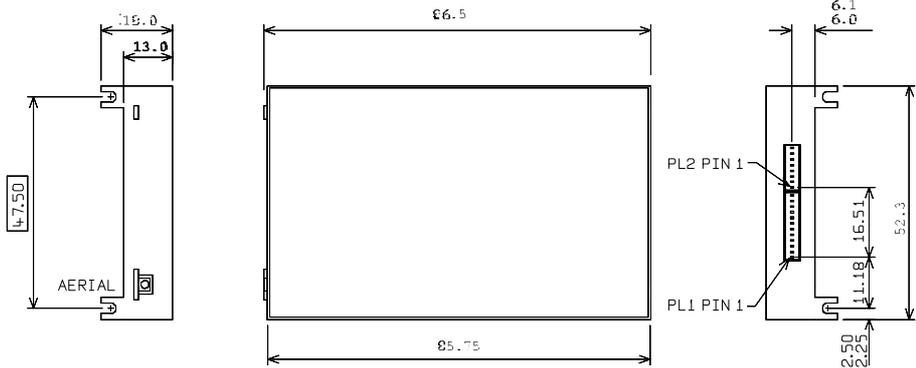
Figure 1 SX150A fixing detail
