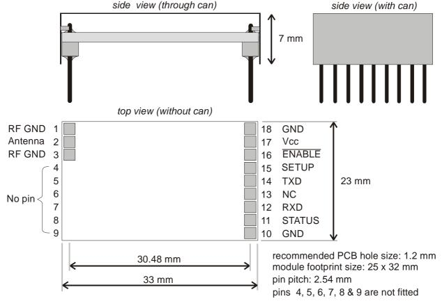
Figure 3: TDL2A footprint (top view)
