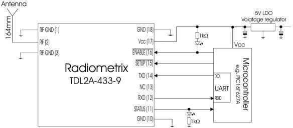
Figure 6: TDL2A interfaced directly to a microcontroller
