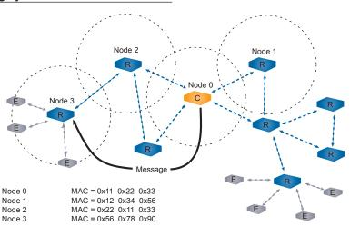
In previous sections (refer to "Mesh Routing (AODV)"), the Ad-Hoc On-Demand Vector routing protocol, Route Requests and Replies were discussed. Fortunately, the routing, RREQs and RREPs are not left up to the OEM Host and are all taken care of by the ZigBee protocol embedded in the ZB2430. A message can therefore be sent to a device anywhere on the network once its 16-bit NWK address is known.
