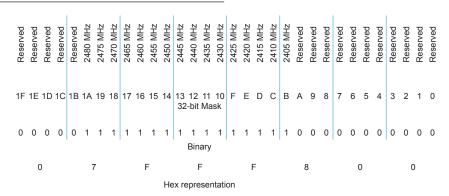
The example in the graphic below shows channels 0x14-0x1A as the only available channels to select from.
