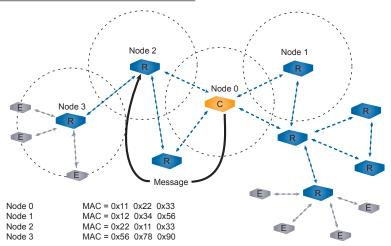
Next, assume that Node 1 needs to send a message to Node 2, which is also out of its range. The procedure is the essentially the same as in graphic above. Note that the underlined values will vary from radio to radio.
