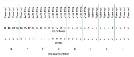
Finally the following graphic shows channels 0x0B-0x10 as the only available channels to select from.
