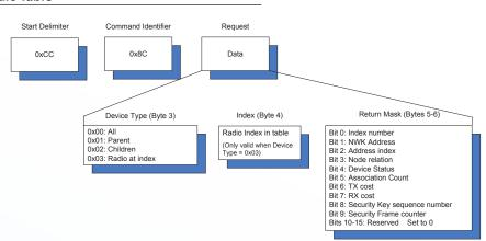
After issuing the Read Radio Table command, the radio will respond with the requested information as shown in the following graphic. The actual command response format may vary depending on the Return Mask setting used in the command.
