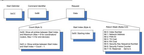
After issuing the Read Neighbor Table command, the radio will respond with the requested information as shown in the following graphic. The actual command response format may vary depending on the Return Mask setting used in the command.
