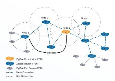
Since Node 0 cannot directly communicate with Node 3, it sends out a RREQ, which is heard by Nodes 1 and 2.
